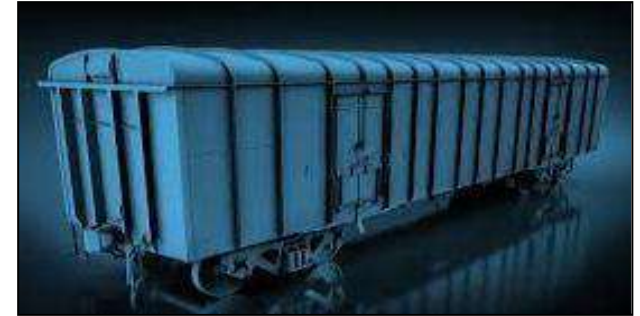
BRN Wagons for Steel Rails and Flats
