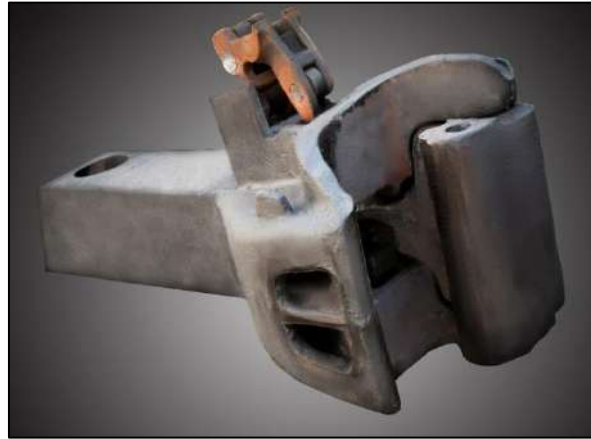
Passenger Coupler with balance Draft Gear
